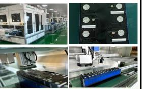
Fully Automatic Battery Soft Plate Laser Welding Technology
